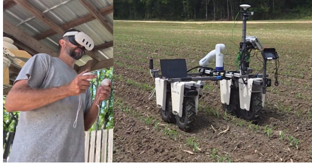
Figure 8: Field test with on-demand remote teleoperation
